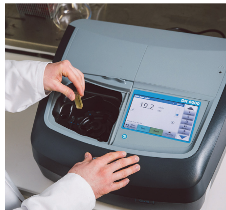
Fig 2. FAN Measurements with a DR6000 UV-VIS Spectrophotometer
